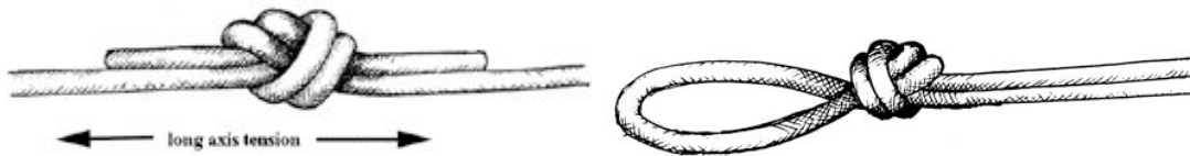
A bend and a loop stressed along their long axes - correct applications in each case
